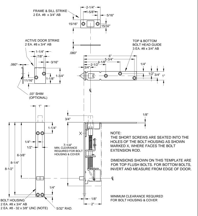
SCREW DETAILS: #8 - 32 x 3/8" UNC - FLAT COUNTERSUNK HEAD MACHINE SCREW, TOTAL 2 PCS. #8 - 32 x 3/4" AB - UNDERCUT FLAT COUNTERSUNK HEAD, DUAL PURPOSE MACHINE/TAPPING SCREW, TOTAL 6 PCS. #10 - 32 x 3/4" AB - FLAT COUNTERSUNK HEAD TAPPING SCREW, TOTAL 3 PCS.
